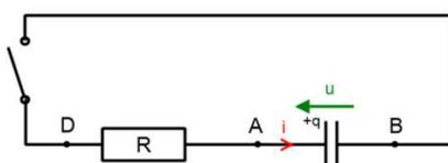
$$u + RC \frac{du}{dt} = 0 \quad (1) \quad u(t) = A + Be^{-\frac{t}{\tau}} \quad \text{donc} \quad \frac{du}{dt} = -\frac{B}{\tau} e^{-\frac{t}{\tau}}$$
